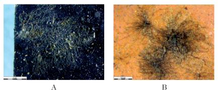
**Fig. 2.** Growth of micromycetes on the surface of samples of low viscosity rubber compound (A) and thiokol sealant (B)
